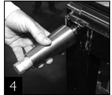
4 Thread leg into cabinet bottom frame rail.
