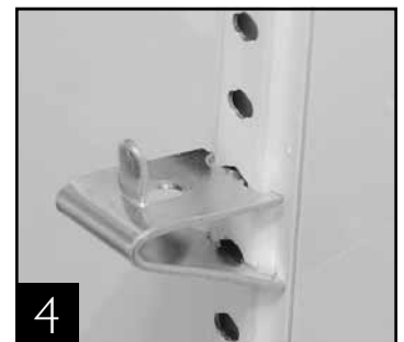
4 Shelf clip installation complete
