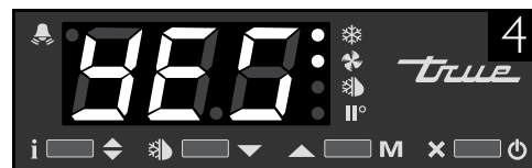
Image 4: If "yes" appears on screen, the controller is locked.
