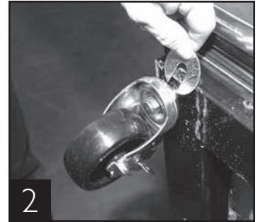
2 For leveling, insert the shim between castor and frame rail.
