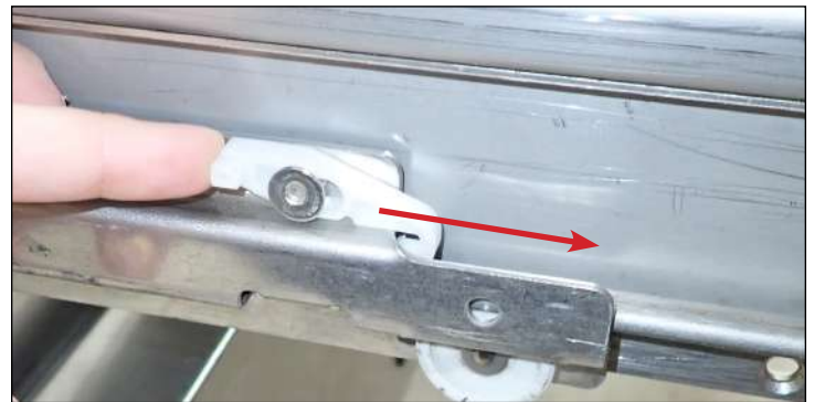
Fig. 2a. Push the retainer forward.
