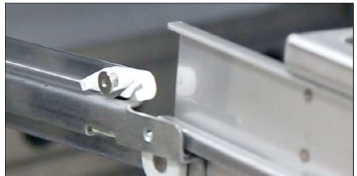
Fig. 3. Align the drawer with the drawer slide.
