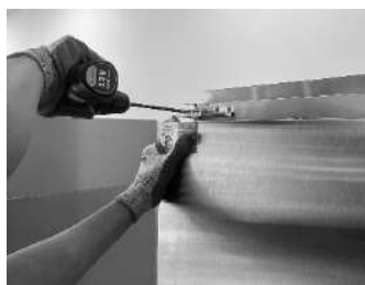
H. Assemble the hinge, then place the hinge into the hole on the inside
