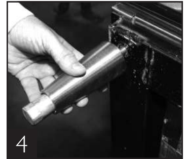
4 Thread leg into cabinet bottom frame rail.
