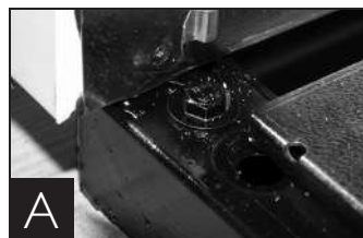
Removing skid from bottom of cabinet.
