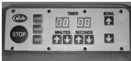
Power Bowl Lift, Mode & Timer Controls (Models SP62P and SP80PL)
