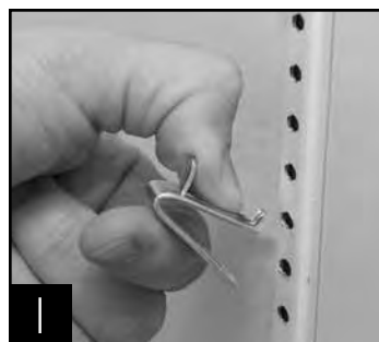
1 Installing top tab of shelf clip
