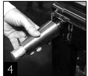
4 Thread leg into cabinet bottom frame rail.
