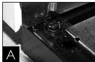
Removing skid from bottom of cabinet.
