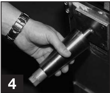
4 Thread leg into cabinet bottom frame rail.
