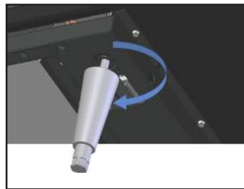
Fig. 4. Screw in the leveling legs.
