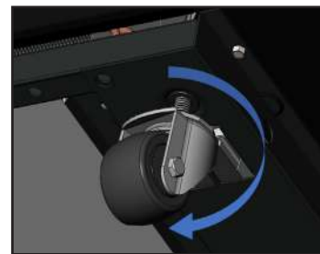
Fig. 8. Position multiple shims at 90° angles.
