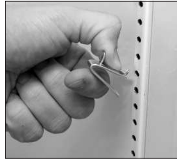
Fig. 1. Installing top tab of shelf clip.
