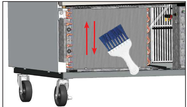
Fig. 4. Never brush across the coil fins.
