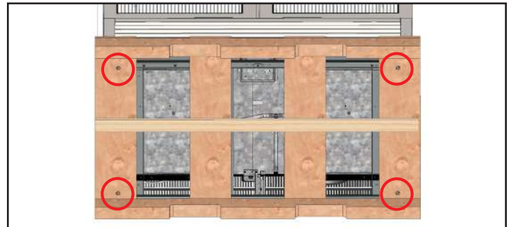
Fig. 4. Shipping bolt locations.
