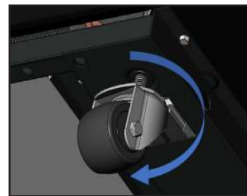
Fig. 8. Position multiple shims at 90° angles.
