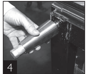
4 Thread leg into cabinet bottom frame rail.
