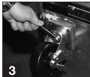
3 Use the tool provided to tighten the castor into place.
