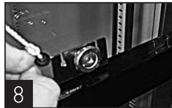
Door roller bracket with nylon cord.
