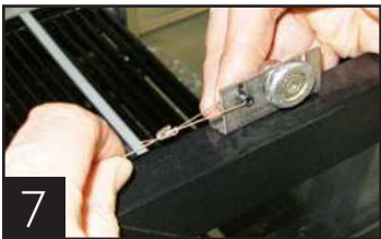
Door roller bracket with metal cable.
