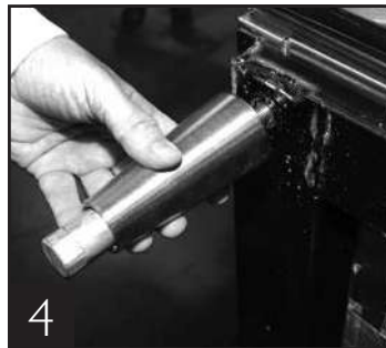
4 Thread leg into cabinet bottom frame rail.
