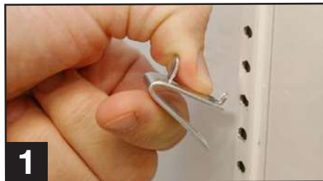
1 (Installing top tab of shelf clip)
