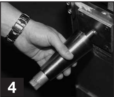
4 Thread leg into cabinet bottom frame rail.
