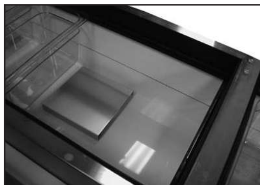
Baffle in the correct location.
