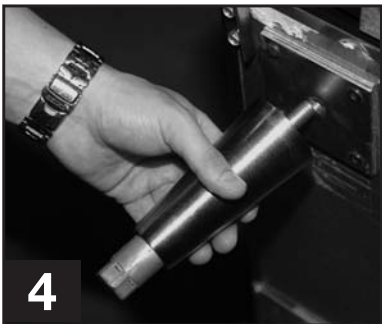
4 Thread leg into cabinet bottom frame rail.
