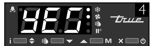
Image 4: If "yes" appears on screen, the controller is locked.
