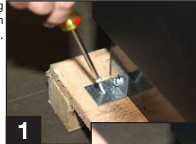
Removing bracket from cabinet.
