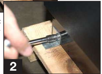
Removing bracket from cabinet.
