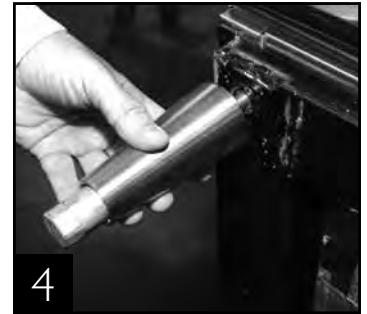
4 Thread leg into cabinet bottom frame rail.
