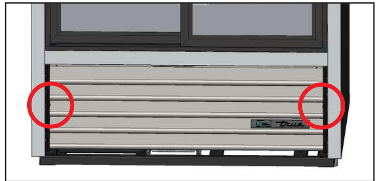
Fig. 2. Slide door louver grill screw locations.
