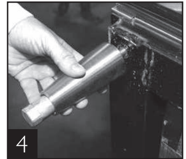
4 Thread leg into cabinet bottom frame rail.
