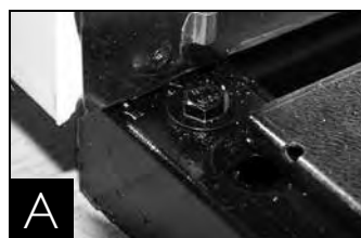
Removing skid from bottom of cabinet.
