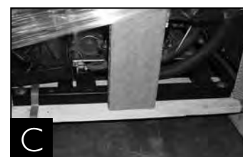
Removing skid from bottom of cabinet.
