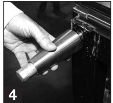
4 Thread leg into cabinet bottom frame rail.
