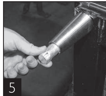
5 The end of the leg is adjustable for easy leveling.
