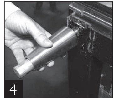
4 Thread leg into cabinet bottom frame rail.
