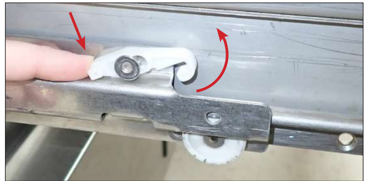
Fig. 2b. Push the back of the retainer down.
