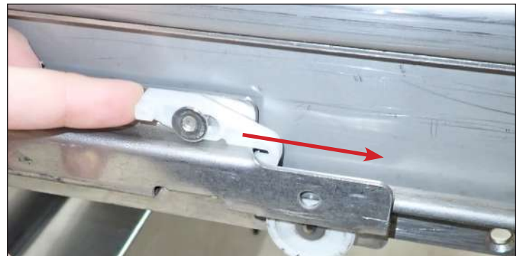
Fig. 2a. Push the retainer forward.
