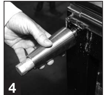
4 Thread leg into cabinet bottom frame rail.
