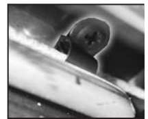
P-Clip keeps cord in-place (prevents cord damage).
