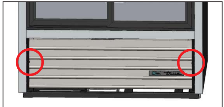
Fig. 2. Slide door louver grill screw locations.
