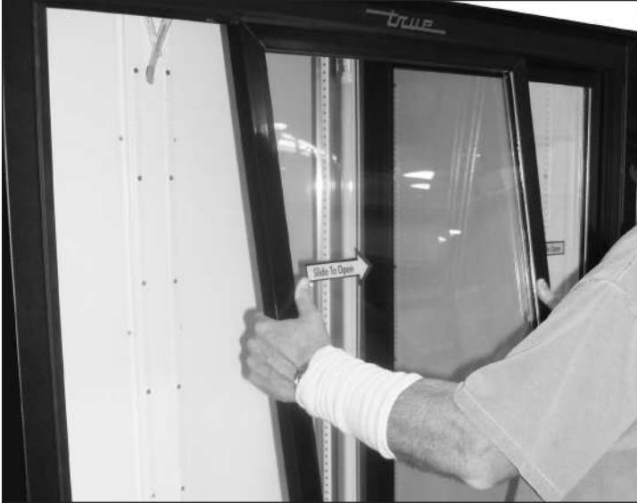
Fig. 4. Carefully remove the door.
