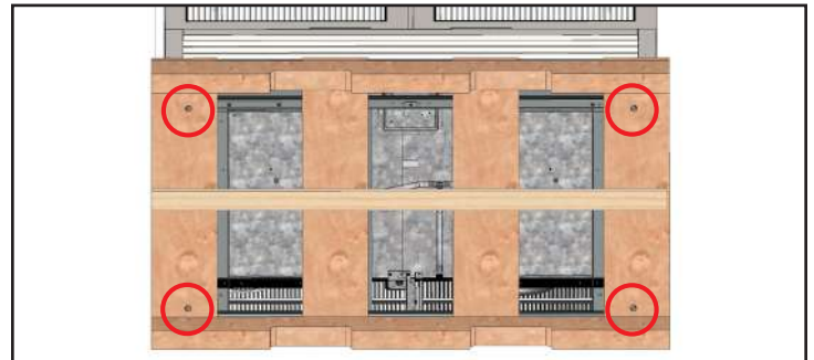
Fig. 4. Shipping bolt locations.
