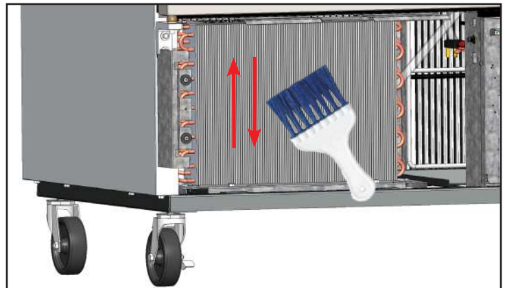
Fig. 4. Never brush across the coil fins.
