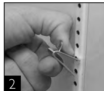
2 Installing bottom of the shelf clip
