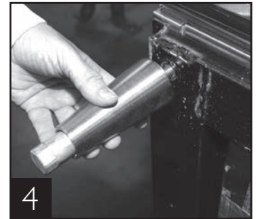
4 Thread leg into cabinet bottom frame rail.
