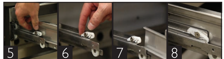
4 Shelf clip installation complete
