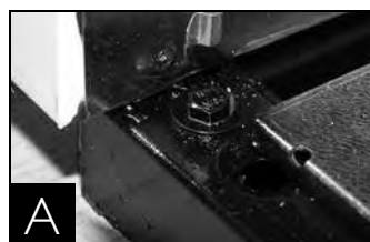
Removing skid from bottom of cabinet.
