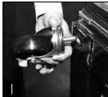
1 Thread castor into the underside of cabinet frame rail.
