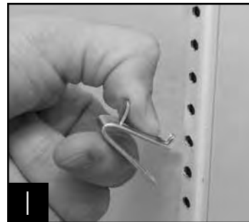
1 Installing top tab of shelf clip
