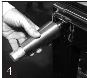
4 Thread leg into cabinet bottom frame rail.
