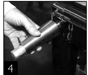
4 Thread leg into cabinet bottom frame rail.
