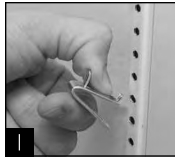
1 Installing top tab of shelf clip
