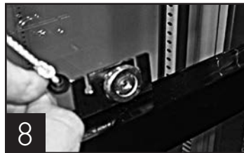
Door roller bracket with nylon cord.
