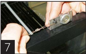
Door roller bracket with metal cable.
